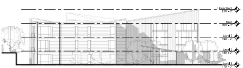
3 Exterior - East Elevation 1/16" = 1'-0" 0 4 8 12 16 24 32 48 (ft)
